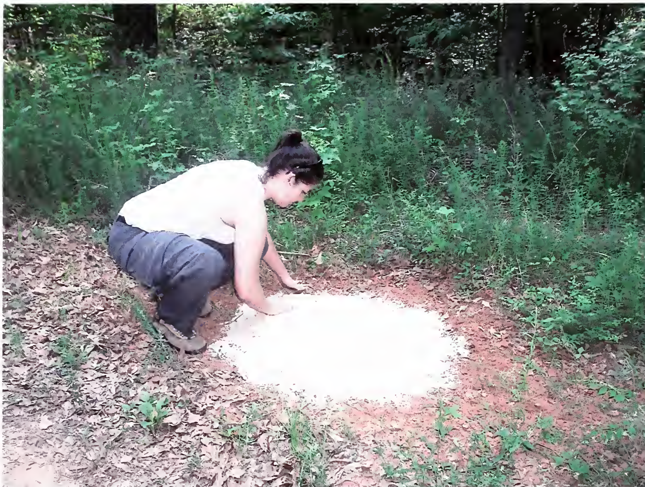
Figure 15. Sand and mineral oil mixture being leveled.
